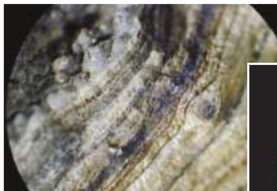
Struvite (Magnesium-Ammonium-Phosphate) in combination with sludge/polymer deposits.
